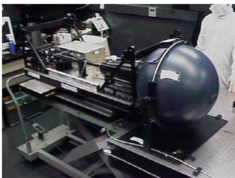
NASA calibration rely on GSFC integrating sphere.
