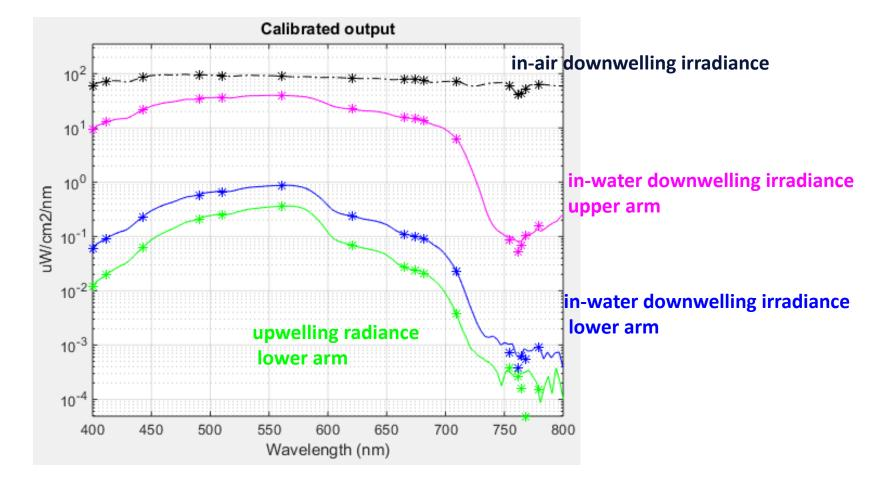
Background subtracted and calibrated output radiometrically calibrated for wavelength and response. Stars represent radiometric value after spectrum response functions (SRF) have been applied for each satellite band. (Downwelling irradiance lower arm temporarily out of commission.)
