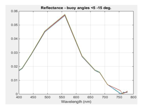
Reflectance calculated on same data with different platform tilt angle tolerances. Variation in varying the acceptance of data from  $\pm 5^{\circ}$  to  $\pm 15^{\circ}$ .
