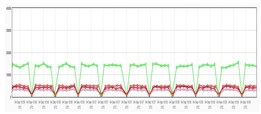
Acquisition sequence for 4 HyperOCRs taken from CoastEye archives. Note: Every 5 light frames is followed by a dark frame simultaneously across all sensors. (Levels are taken by averaging their respective spectra around 500 nm).
