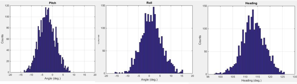
Pitch, roll, heading over 10 min interval with no tidal effects
