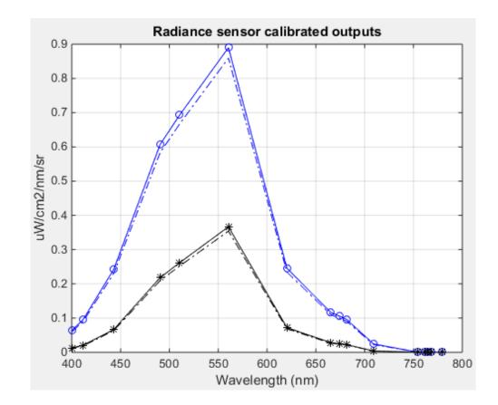
Upper and lower radiance sensors with selfshading correction applied (solid line with circles/stars)
