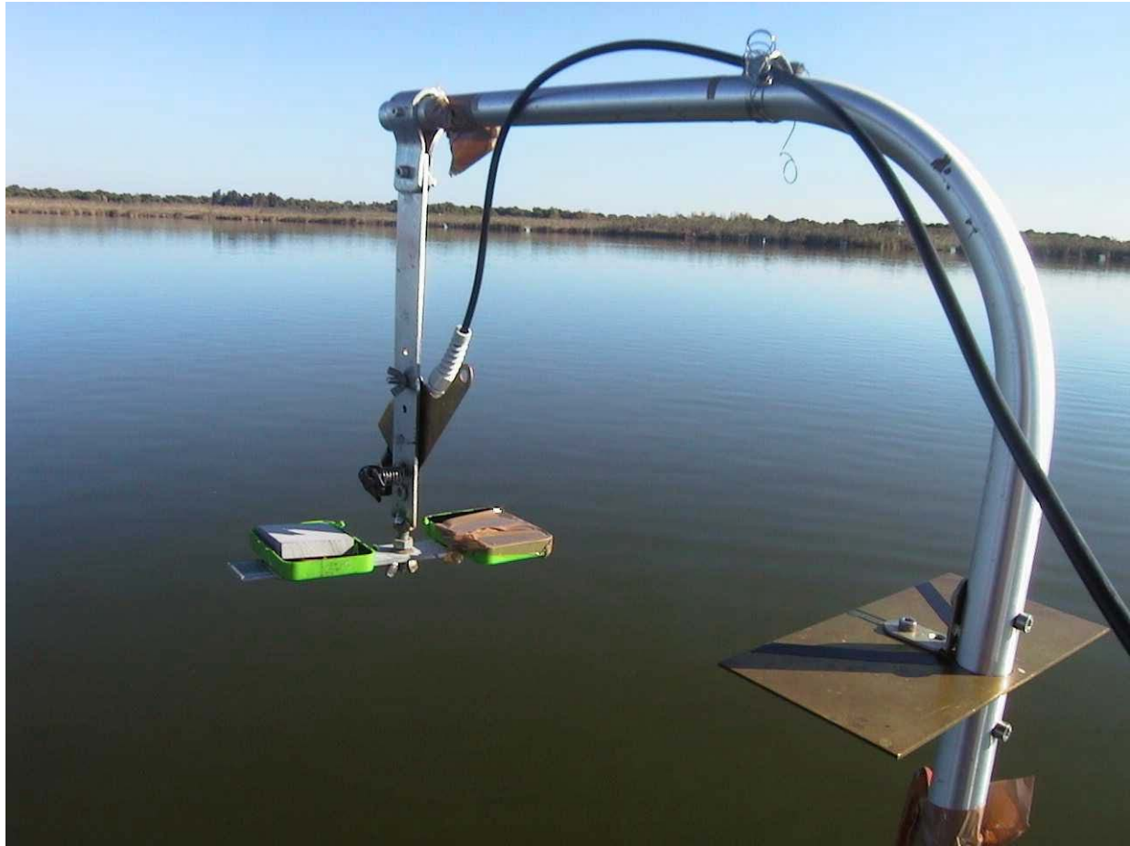
Figure 3-8 Typical measurement equipment and deployment for measurement of E_d^{0+} using a downward pointing radiance sensor and a reflective plaque. Photo courtesy A. Ruiz-Verdu.
