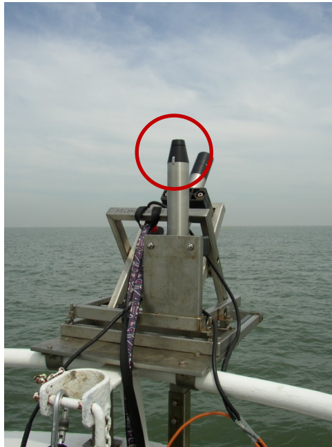
Figure 3-2 Typical deployment of above water irradiance sensors (top) Combined with a sunphotometer system on a mast, taken from (Hlaing et al. 2010) (bottom) combined with sea- and sky-viewing radiance sensors at the prow of a ship, as in (KG Ruddick et al. 2006)
