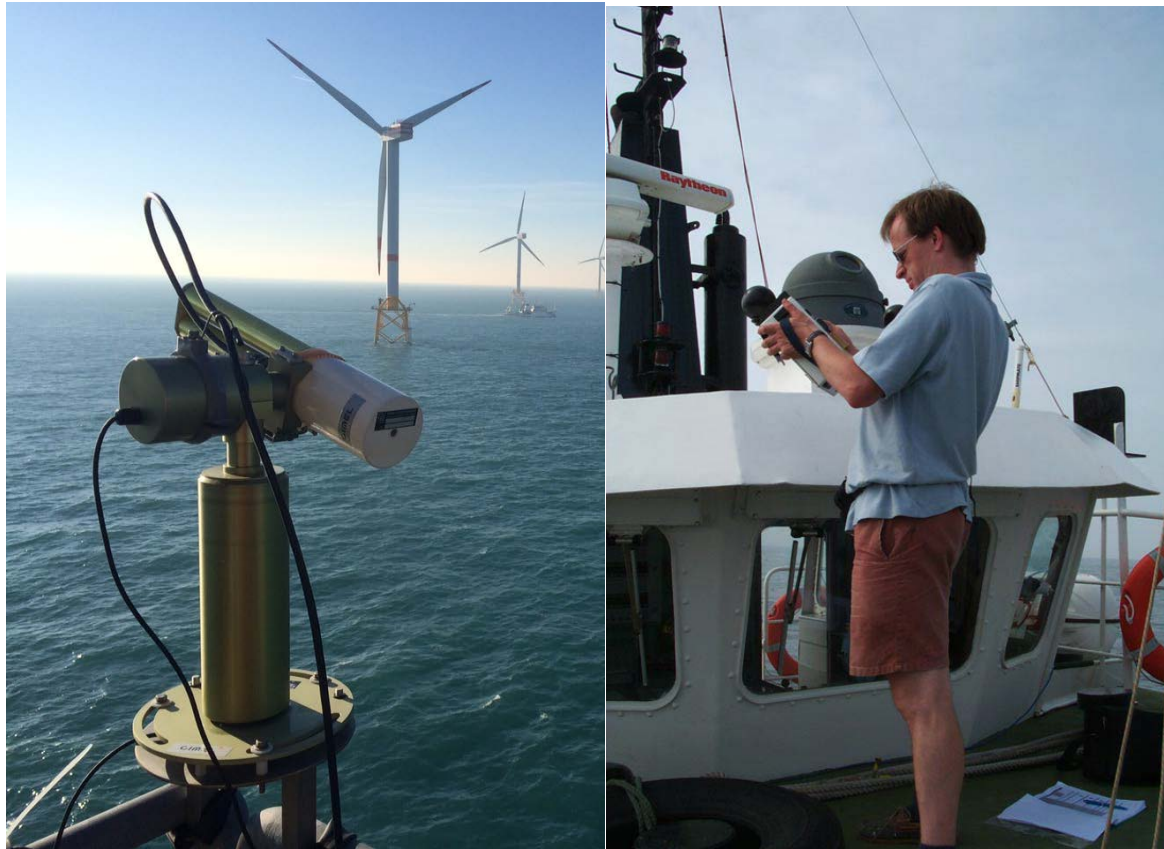
Figure 3-6 Typical deployment of instrumentation for estimation of E_d^{0+} by sunphotometry. (left) SeaPRISM instrument [photo courtesy: Dimitry Van Der Zande], (right) handheld SIMBADA instrument.
