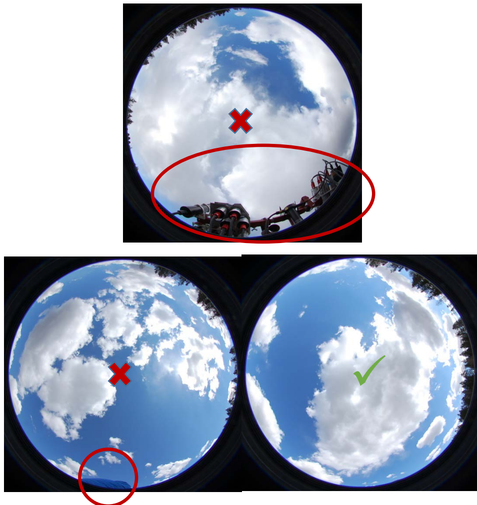
Figure 3-4 Example fish-eye photos taken to check for contamination of E_d^{0+} measurements. (top) Contamination of field of view by other instruments, (middle) Contamination of field of view by a scientist in bottom of photo, (top) No
