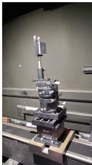
(left) aligning the mirror so that the centre of rotation coincides with the laser
